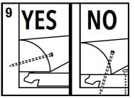
Prior to installing moldings, apply silicone sealant to the portion of the molding or transition that will rest on the laminate flooring surface. Install moldings and immediately wipe away excess sealant. Apply silicone sealant at connections to doorframes and other fixed objects. Ensure floor is able to "float". Do not nail planks or trim to floor.
