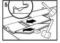
Use a 4"-6" piece at an angle to hold the tongue and the groove on the same plane, limit end-joint damage and ensure planks engage square. Tap end-joints with multiple taps, striking the tapping block evenly until endjoints close. **NOTE: Tapping too hard** or striking the tapping block unevenly can result in installation-related damage or peaking.
