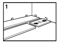
Before cutting, select your beginning wall and plan your installation. Lay planks tongue side facing the wall for the first 2 rows on the floor close to the wall. Each plank should be at least 12" long.
