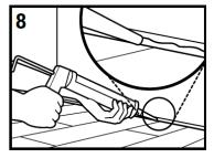
Remove all spacers before installing trim. Create a water tight seal by applying flexible 100% silicone sealant along the perimeter of room and around fixed objects. Do not use acrylic sealant. To reduce the amount of sealant, first fill all expansion spaces with 3/8" compressible PE foam backer rod and cover with silicone sealant.
