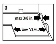
Always allow for 5/16" min to 3/8" max expansion at walls and around fixed objects. A transition strip is required when length or width of installed planks measures 40' and in doorways if plank direction changes.
