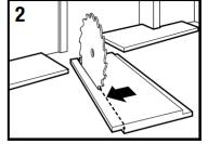
Remove the tongue side (see pictures above) on only the planks in the first row that face the wall to allow room for spacers.
