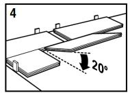
Lock in panel lengthwise. Allow a 12" minimum end-joint stagger row to row. Install first and second row at the same time to help ensure endjoints are perfectly square.
